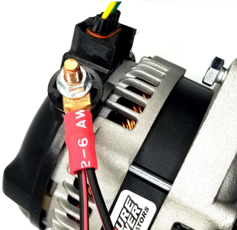
Cut off original B+ charge wire plug as shown, cut back 1" from plug.
